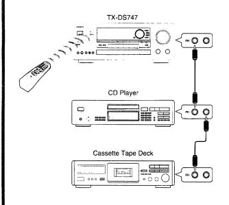
Connect a remote control cable to the black connector with the RI mark. Never connect it to the gray or green connector with the MR mark.
