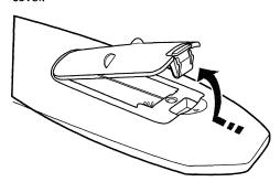
2 Insert two AAA batteries into the battery compartment. Make sure that you match the + and – symbols on the batteries with the + and – symbols in the battery compartment.
