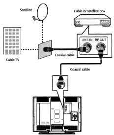
2 Connect a 75 ohm coaxial cable to the RF OUT jack on the cable or satellite TV box, then connect the other end to the ANT. IN jack on the back of your TV.
