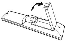
2 Insert two AA batteries into the battery compartment. Make sure that the + and - symbols on the batteries match the + and symbols in the battery compartment.
